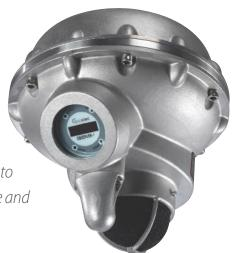
With ANN technology, the GASSONIC OBSERVER-i makes it possible to fully analyze the sound spectrum as low as 12 kHz since common high pass filters are not used. This provides a broader leak detection range which also increases sensitivity to smaller gas leaks, without interference from unwanted background noise.
