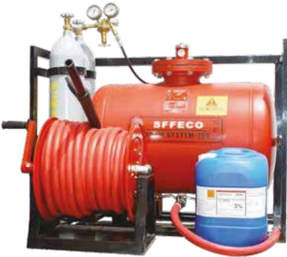
SSFECO Foam system unit is constructed with a heavy duty tank with corrosion proof coating. Two External nitrogen cylinders are provided for pressurizing the tank.
